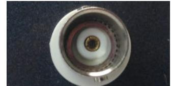
**Caution: the integrator output should only be connected to high impedance recording instruments.**
