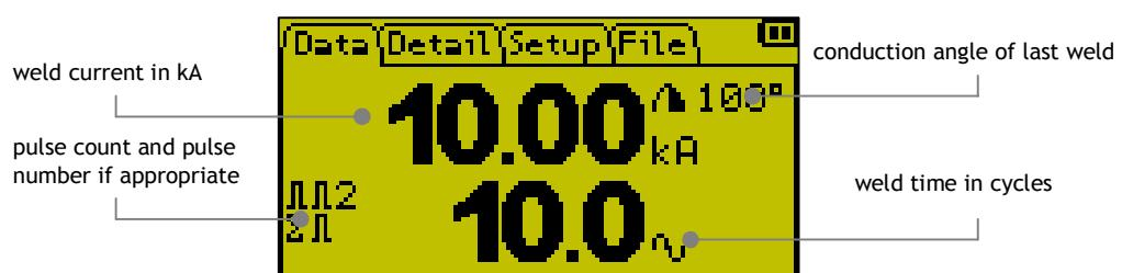
For DC welds, the weld time is shown in ms and cycles. The conduction angle is not applicable to DC welds.
