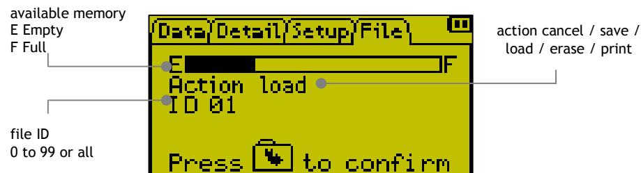
The display shows the memory that is available for storing welds; the value will change according to the quantity and duration of welds that are stored.
